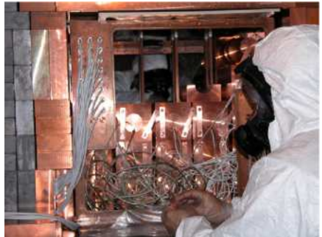
Fig. 6. The installation of the 25 NaI(Tl) crystals (9.70 kg each) of DAMA/LIBRA in high-purity nitrogen atmosphere. All the procedures as well as the photos have been carried out in high-purity nitrogen atmosphere.
